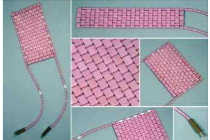
These beads are supplied to us by one of the leading specialist ceramic manufacturers in the ceramic industry. The cold tails of Cooperheat ceramic heating elements are butt welded to the heater core wire which eliminates the cold tail/core wire junction failures often seen with low quality heaters which use steel ferrules.
