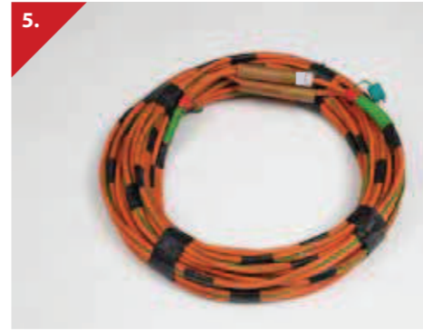
5. Triple cable sets For use with treatment units controlling 30V, 40V, 60V and 80V heating elements. Includes two double insulated cables for power feed and return, fitted with 300A plug and socket connectors and one compensating cable fitted with type K thermocouple plug and socket.
