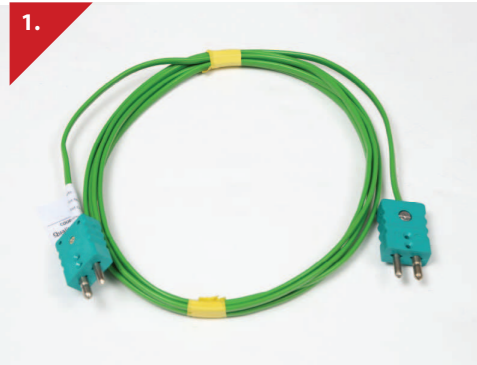
1. Compensating cable link cables To link controller/programmer thermocouple input to the recorder input. Reference & description: 34013 - 3m 'jumper' compensating lead fitted with two type K thermocouple plugs
