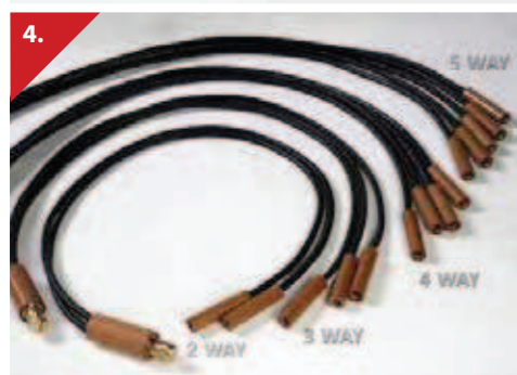
4. Splitter cables For use with triple cable sets. Splitters are used where the operator needs to connect multiple heating elements, in parallel, to triple cable sets to enable the control of multiple heating elements. This enables the heating elements to be grouped to a single control output from a heat treatment unit to allow accurate zonal temperature control. Reference & description: 32001 2 Way splitter 32002 3 Way splitter 32003 4 Way splitter 32004 5 Way splitter
