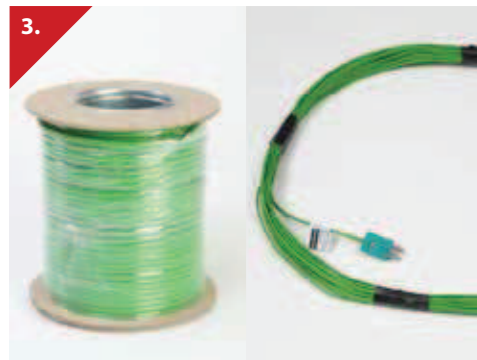
3. Thermocouple compensating cable Suitable for use with type K thermocouples where monitoring thermocouples, in addition to the control thermocouples, are required for temperature monitoring purposes. Available in 30m lengths complete with type K thermocouple plug and socket or in 100m rolls without plug and socket (plugs and sockets can be supplied separately as required). Reference & description: 34000 - 30m compensating cable c/w type K thermocouple plug and socket 504-062 - 100m roll of compensating cable without thermocouple plug or socket
